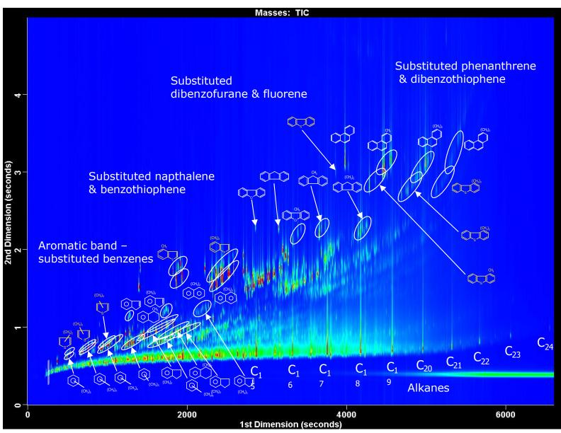
Diesel analysis by direct injection GCxGC-TOFMS
